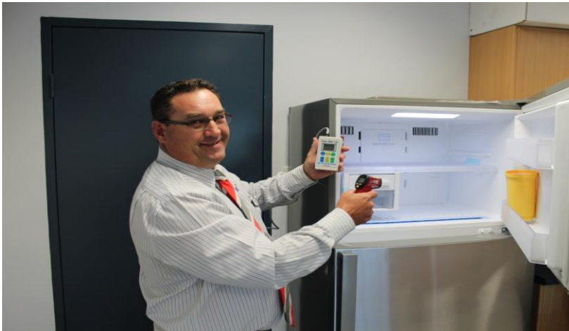
Home Energy Advisor Rob Walters measuring fridge temperature and electricity consumption.
