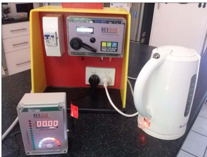
BEEBox demonstration display kit connected to an electric jug
