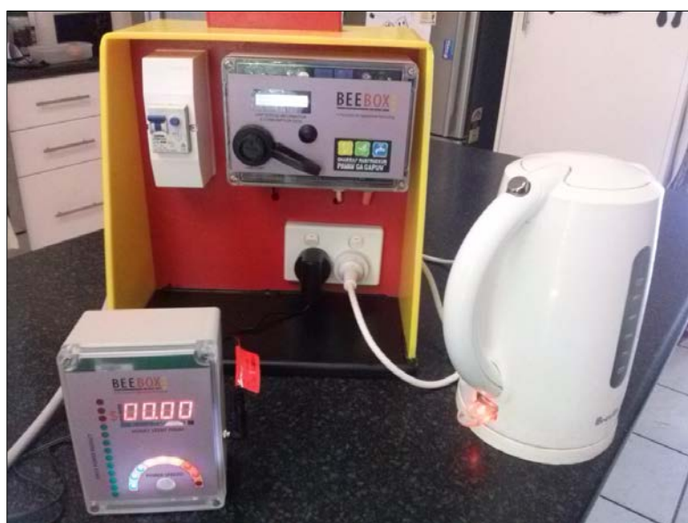
BEEBox demonstration display unit connected to an electric jug
