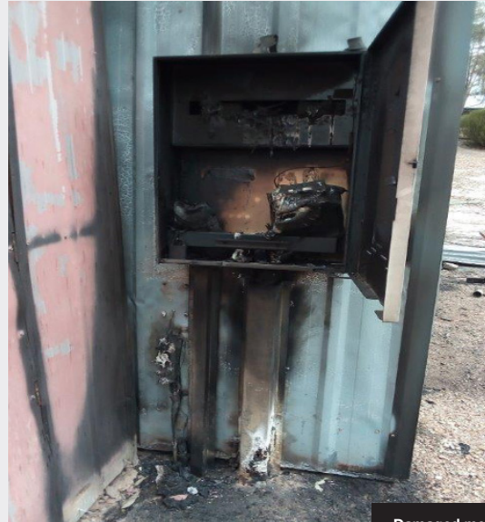
Damaged meter box and call for Electrician. Photo courtesy of Cathy.
